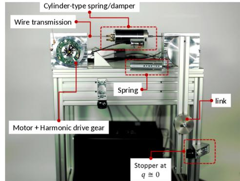
Fig. 7. Experimental setup. The left and right discs (i.e. motor- and link-side inertias, respectively) are connected by a steel cable. A joint module from DLR LWR with 1:100 gear ratio is used. In the transmission, the upper element is explained in Fig. 8, and the lower one is a steel spring. An end-stop is located at  $q \approx 0$ .
