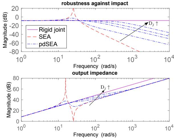
Fig. 2. Top: magnitude bode plot for (1). Bottom: the plot for (2). Physically damped SEA is a combination of SEA and rigid joint robots, but more likely to behave like rigid joint robot, as  $D_j$  grows. This is obvious from physical sense because higher damping makes the joint coupling stronger.
