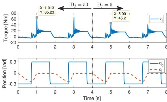
Fig. 10. Experimental result for impact test. To make periodic impact,  $q_d$  was defined as a periodic pulse signal.  $D_j$  was 50, and was changed to 5 at  $t = 4$ s. The measured impact torque was reduced when  $D_j$  was lowered because it weakens the coupling. Namely, the system behaved more like a SEA system.
