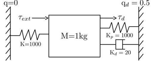
Fig. 4. Motivating example. PD control is applied to the mass  $m$  which is connected with the environment by spring.
