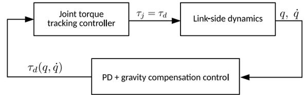
Fig. 1. Overview of the control scheme. Inner-loop joint tracking torque control is cascaded by the outer-loop PD controller.
