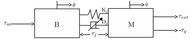
Fig. 3. Schematic diagram of VPDA.  $M$ : Link-side inertia,  $B$ : Motor-side inertia,  $\tau_m$ : motor torque,  $\tau_j$ : joint torque,  $\tau_g$ : gravity torque,  $\tau_{ext}$ : external torque acting on the link inertia,  $K_j$ : joint stiffness,  $D_j$ : joint damping,  $\theta$ : motor position, and  $q$ : link position.
