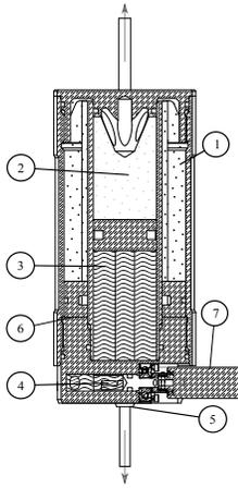
Fig. 8. Cross section of the VPDA with an elastic element formed by the active air chamber (1) and the linearizing air chamber (2), connected by the hydraulic system (3)(6) with the variable throttle valve (4) providing viscoelastic behavior on the piston rod (5). A mini servo (7) sets the damping throttle.
