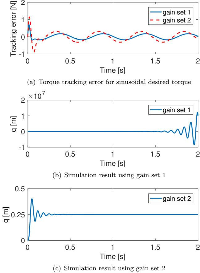
Fig. 5. Simulation result for the motivating example. Both sets of gains tracks sinusoidal test input reasonably. However, when the PD control and environmental interaction is considered as shown in Fig. 4, the gain set 1 did not stabilize the system, whereas the gain set 2 stabilized it.
