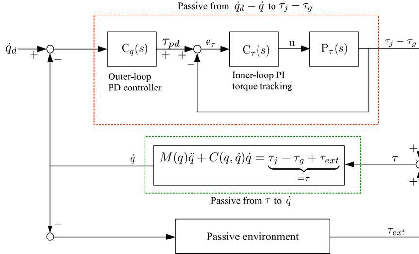
Fig. 6. Overall control structure. If the upper part (red dotted) is passive from  $\dot{q}_d - \dot{q}$  to  $\tau_j - \tau_g$ , then the overall control structure can be constructed by feedback interconnections of passive subsystems.  $C_q, C_\tau, P_\tau$  are defined by (17).
